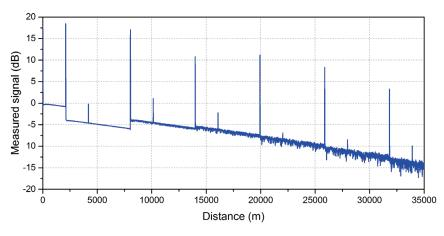
By analyzing the resulting signals, DFM can calibrate the OTDR distance scale over many kilometres of optical fibre and enable the location of faults to be found with high precision.
