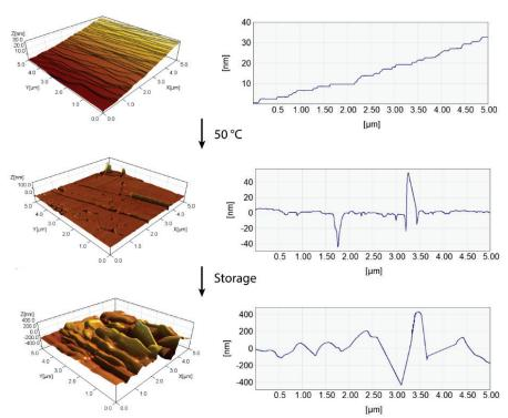
The example shows how AFM monitored the surface structures of a crystal hydrate. At first, the crystal in the upper figure was dehydrated due to exposure to raised temperature. Then, the crystal was rehydrated over time during storage at ambient conditions.
