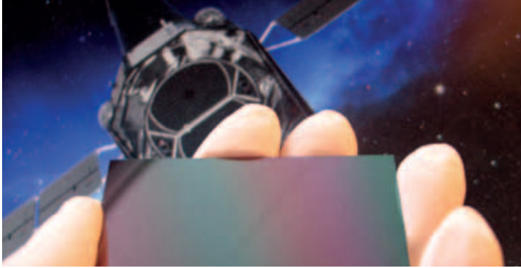
Silicon substrate for X-ray mirrors. The background image (from ESA, sci.esa.int ) is an artist's impression of the ATHENA spacecraft, which is a candidate for a coming ESA mission.
