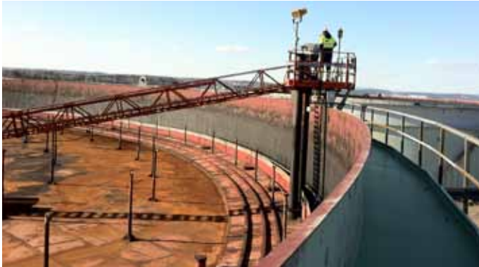
Accurate measurement of large scale facilities is a challenge at e.g. petroleum storage sites. The tank has a diameter D=52\text{m} and height h=16\text{m}
