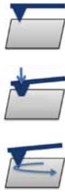
Figure 4. Nanoindentations in a crystal. First the hard tip is pressed into the surface. Secondly the surface is scanned. The image to the left shows the measured imprints. The applied force of the indenter is increased from the right column to the left column; the applied forces are the same in each column.
