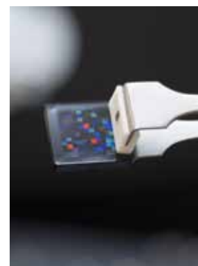
Figure 3. A nano-textured surface, developed in the NanoPlast project, gives the plastic brick an iridescent effect also known from the wings of a butterfly. The nano-textures helps to minimize the use of chemical dyes
