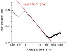
The figure shows a typical Allan Deviation (ADEV) plot for a Stabiλaser 1542.
