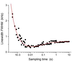
The Stabiλaser 1542 linewidth vs. sampling time. Fourier limited at short times.
